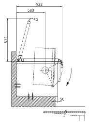
Cold Water inlet 1 (cleaning) FΙ Electrical inlet (power) HWI Hot water inlet
